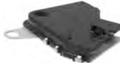
NS6569 Neutral Safety Switch 1994237, 1994245, 1994253, D2201A Usage includes Back-Up Light, Neutral Safety
