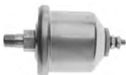
OP6743 Oil Pressure Switch Gauge Type, 1/8 x 27" thread, 10-32" stud terminal, 100 PSI system, for Single Station.
