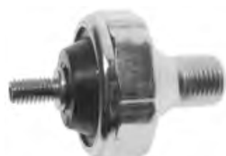
OP6741 Oil Pressure Switch Gauge Type, 1/8 x 27" thread, 10-32" stud terminal, 15 PSI system. Also used as Fuel Pump Shut-off.
